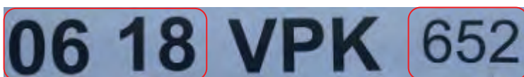
Figure 2: Sample tank inspection markings, highlighting the date of inspection (06 18) and inspector Transport Canada Registration Number (652)
