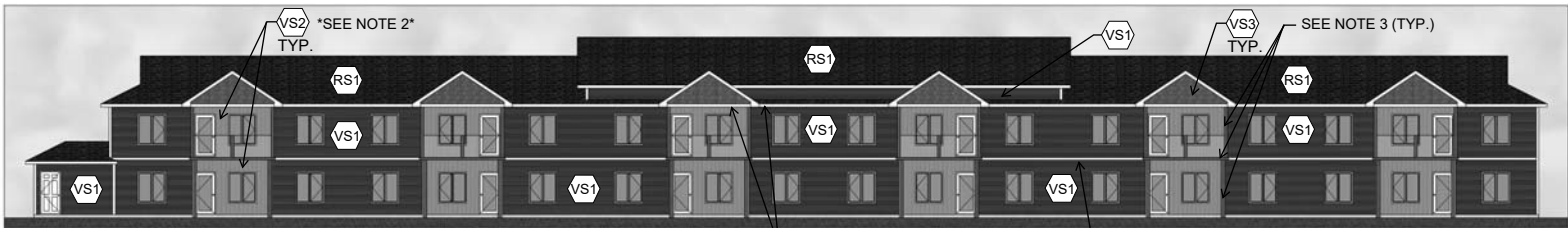
REAR ELEVATION SEE NOTE 4 (TYP.) HORIZONTAL TRIM TO MATCH FINISH/PROFILE OF CORNERS & TO LINE UP WITH DECKS AS SHOWN (TYP.)
